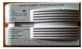
Each RV is equipped with a propane detector, which is always located near the floor. The alarm goes off whenever an increased propane emission (e.g. from the stove or oven) is detected. Please do not to place any objects near the propane detector to avoid false alarms.
